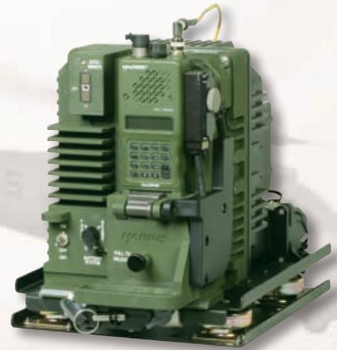
**The RF-300M-HV 102 provides power amplification, battery charging, and a shock mount—all in a compact package.**
