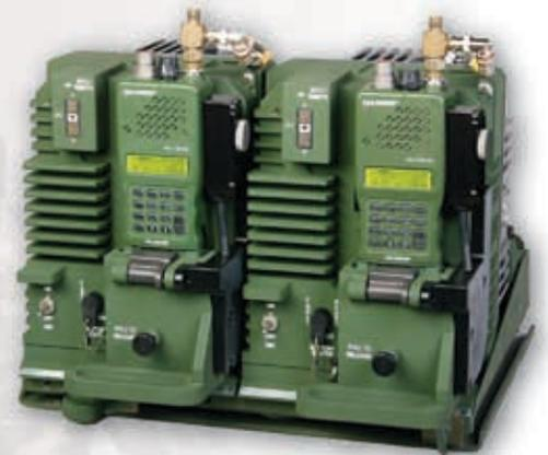
**SINGARS solutions like the AN/VRC-110 shown above provide high power 50 W vehicular communications with the flexibility for multiband and dismounted operations.**
